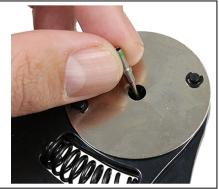
5 Once the four prongs have released from the terminal, remove the terminal and inspect it.
