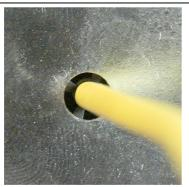
3 Insert the stripped wire all the way into the terminal. Make sure there are no stray strands.
