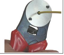
2 Insert the contact into the barrel terminating end first. Use the adjustment screw to make the receiving end flush with the plate.
