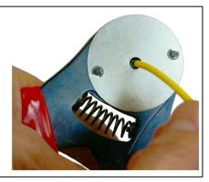
6 Gently pull on the terminal to ensure the crimp is secure.
