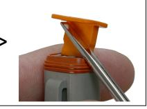
To remove contacts from a connector, first remove the wedgelock (see instructions above). Then use the flat end of the tool to depress the terminal's locking tab while pulling the wire out through the back of the connector.
