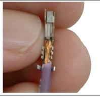
6 Gently slide the wire back and forth to ensure that the terminal is locked in position.
