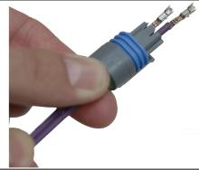
3 Set the stripped wire strands inside of the terminal's inner straps. Make sure the wire's insulation sits inside of the outer straps.
