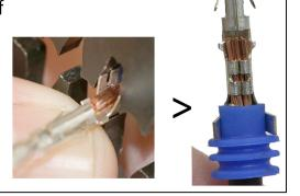
2 Strip 1/4" of wire. Slide the cable seal up to the end of the wire's insulation.
