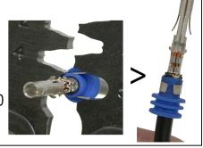
Insert the stripped wire into the terminal's inner straps. Make sure the smaller end of the cable seal rests inside of the larger straps.
