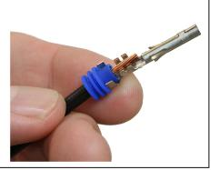
6 Gently pull on the terminal to ensure the crimps are secure.
