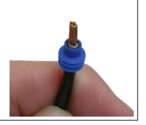
5 Place the cable seal inside the appropriate cavity and squeeze tightly to crimp the cable seal onto the wire's insulation.
